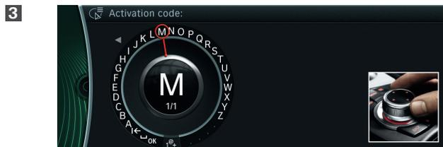
Enter the 20-character **activation code** using the **iDrive controller**. The activation code **does not contain** the digits "0" and "1" in order to prevent confusion with the letters "O" and "I".
