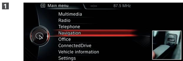
Connect the **32GB USB stick** to the system. The screen display automatically changes to the navigation update mode.
