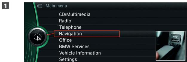
Connect the **8GB USB stick** to the system. The screen display automatically changes to the navigation update mode.
