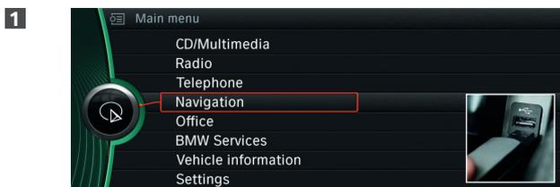
Connect the **16GB USB stick** to the system. The screen display automatically changes to the navigation update mode.
