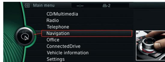
Using the **iDrive controller**, select Navigation in the main menu and press the iDrive controller down once. Select the shortcut button "Options".
